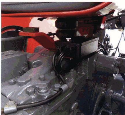
Above and right: part of the all-new electrics. All cables from the rear of the tractor were combined in a single cable-splice box beneath the seat.
